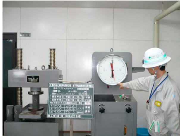
Photo 96 Quality inspection of strength (28 day)
