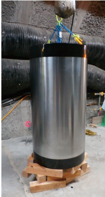
Photo 21 Insulation paint for body of simulated OP (using Duralco 4525 IP)
