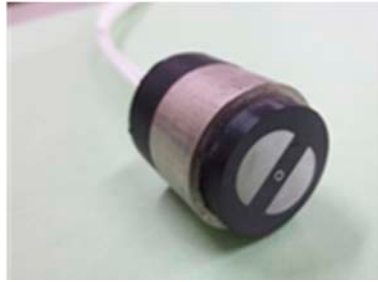
Photo 27 Carbon steel corrosion sensor
