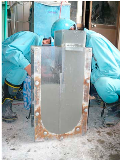
Photo 92 U-shaped filling test
