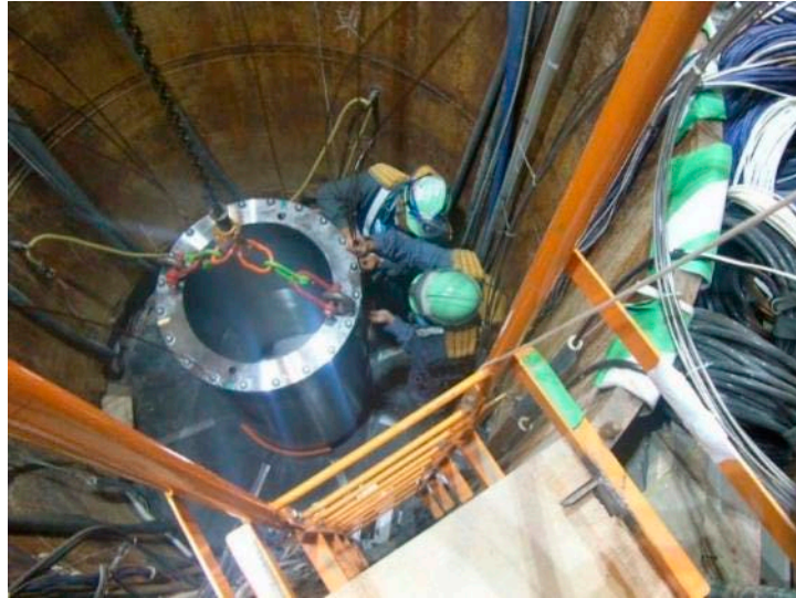
Photo 52 Setting thermocouple on surface of simulated OP
