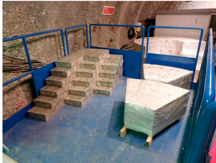
Photo 123 Exhibition of backfilling material blocks
