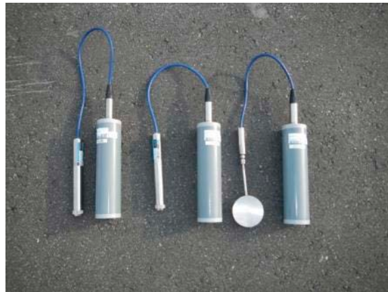
Photo 33 Wireless sensor (piezometer and pressure cell)
