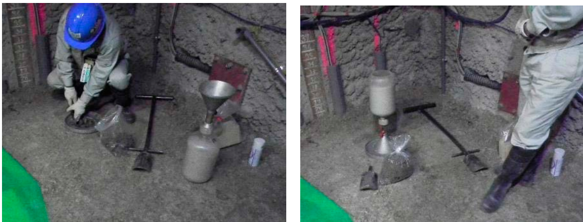
Photo 72 Sand replacement method (Layer No.27, Point A-R)
