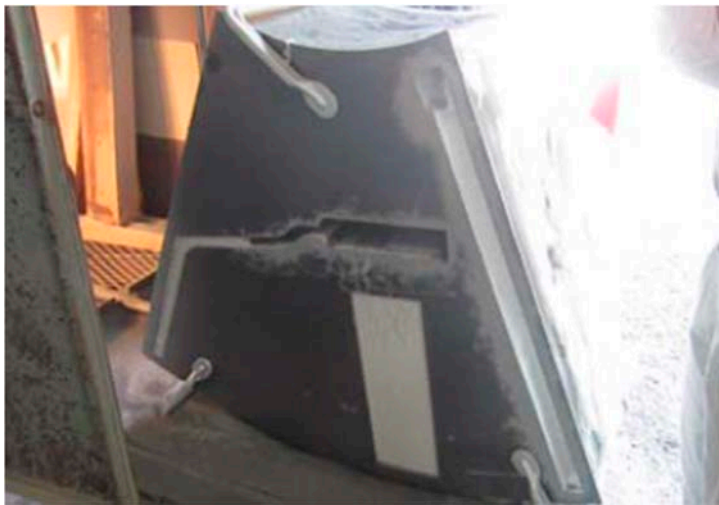
Photo 37 After sandblasting block
