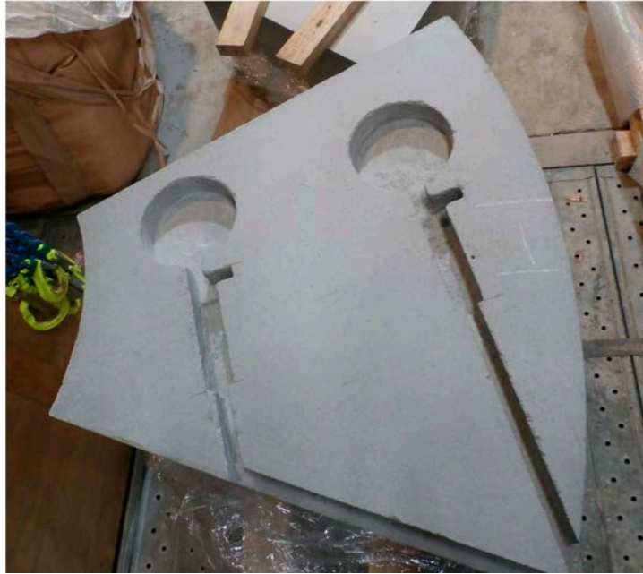
Photo 38 Chased buffer material block for sensor (pressure cell)
