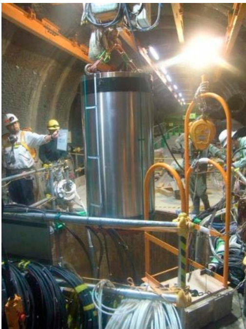
Photo 51 Move simulated OP into test pit
