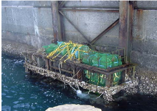
Figure 2.2.6-7 Exposure test under marine condition with HFSC reinforced concrete
