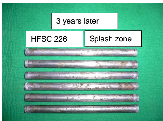
Figure 2.2.6-9 Corrosion status of reinforcing bar embedded in HFSC226 concrete 3 years later
